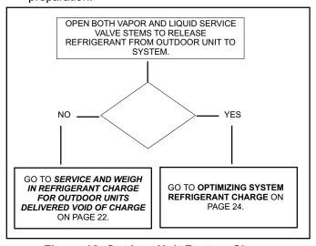
Figure 16. Outdoor Unit Factory Charge
